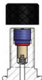
Model of valve stem integrated 7/8"14 UNF (C)
