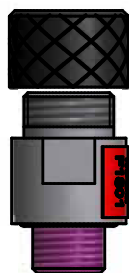
Model of valve stem 5/8" 18 UNF (A)
