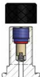
Model of valve stem integrated 7/8"14 UNF (C)
