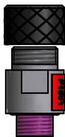
Model of valve stem 5/8" 18 UNF (A)
