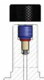
Model of valve stem integrated 5/8" 18 UNF (D)
