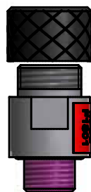
Model of valve stem 5/8" 18 UNF (A)
