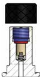
Model of valve stem integrated 7/8"14 UNF (C)
