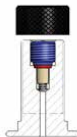
Model of valve stem integrated 5/8" 18 UNF (D)
