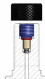
Model of valve stem integrated 5/8" 18 UNF (D)
